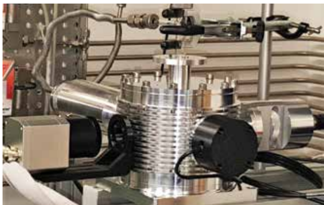
▲ Figure 3. A microwave reactor created by researchers at the Univ. of Delaware (UD) and the United Technologies Research Center could help utilize microwave heat for multiple industrial processes, including hydrogen production and shale gas processes. Image courtesy of UD.
