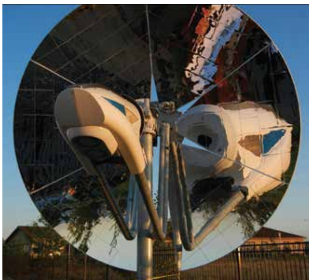
▲ Figure 4. The STARS Technology Corp. uses a unique system to convert solar energy into hydrogen in an energy-efficient manner. CEO Bob Wegeng is working with researchers to streamline the process for commercialization of STARS Tech. Image courtesy of Pacific Northwest National Laboratory.
