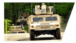
**REDUCING HIGH MOBILITY MULTIPURPOSE WHEELED VEHICLE ROLLOVERS:** This pilot project retrofit Michigan National Guard vehicles with Ricardo Defense System's optimized antilock braking system and electronic stability control to reduce High Mobility Multipurpose Wheeled Vehicle fatal rollovers. The system is now available for purchase by military units worldwide.
