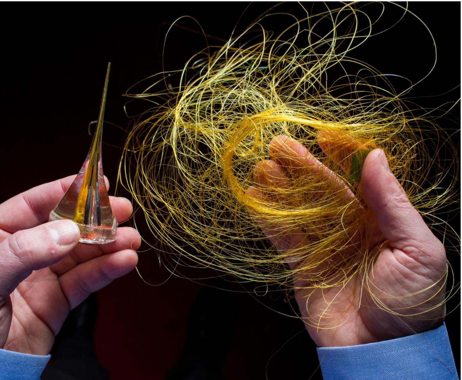
Figure 28. Fibers drawn from a preform that contains semiconductors. By adding computer properties to fabrics, a whole new world of devices could emerge. Credit: M. Scott Brauer; courtesy of AFFOA
