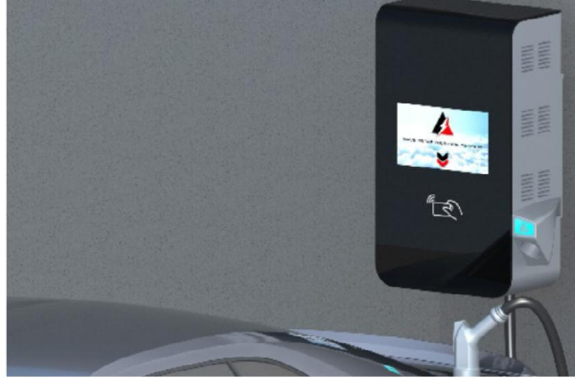
Figure 30. Computer-aided design of an electric vehicle charger designed by NC State University as part of a PowerAmerica project. Credit: NC State University
