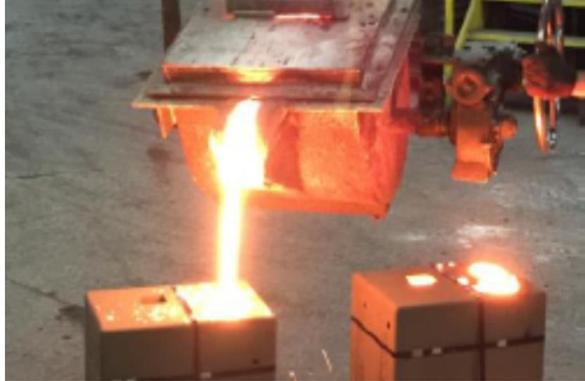
Figure 13 Pouring Iron Into Castings of Differential Housing Used in Heavy Trucks. Credit: LIFT
